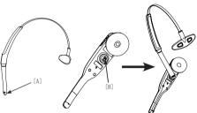
4. Adjust the head band to fit your head. Adjust and rotate the angle of the headset until the microphone is pointing towards your mouth. Firmly grip the earpiece with one hand whenever adjusting the headset microphone up or down.
